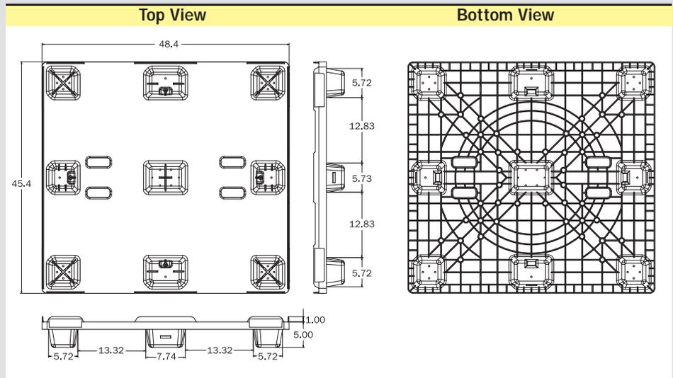
Though Krypto-Lite is shown, above dimensions apply to both the Krypto-Lite and AF Pallet.
