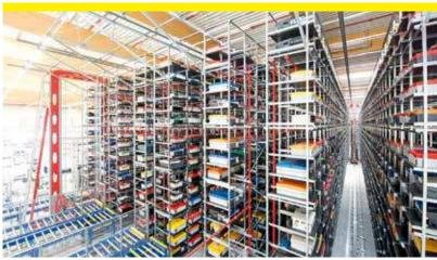
The sophisticated construction of the SMC is geared toward providing the maximum value for the customer. The use of premium steel guarantees high durability and contingency reserves with low costs. Due to the diagonal bracing of the mast, a lower weight, greater elevation and higher throughput are achieved. The design is unique and significant. The traveling unit made with steel-rail and the successful Omega-drive are designed for high availability and low wear.
